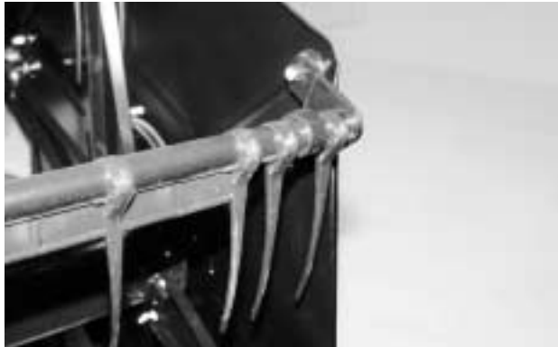
Illustration 11. Bat assembly (the end shields shown in this photo should not be assembled at this time).
