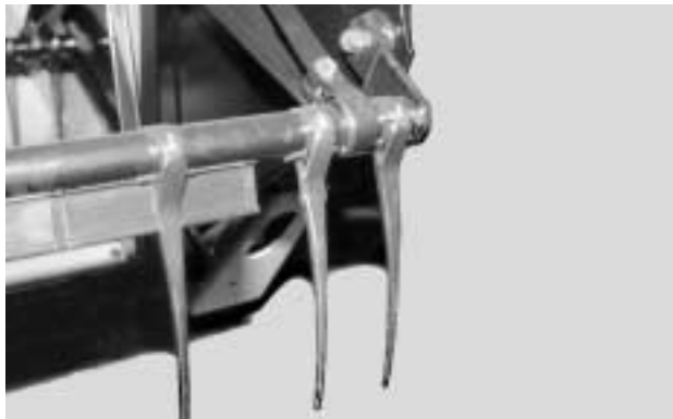
Illustration 12. Bat assembly with alternate tine spacing to bat assembly shown in Illustration 11 (the end shields shown in this photo should not be assembled at this time).
